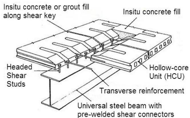
Fig. 2. Structural mechanism between HCU and steel beams, adapted from [2.1].
