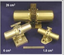
Cryocoolers of different sizes
