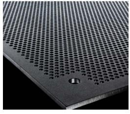
Fig. 2. Perforated Super Bainite armour†
