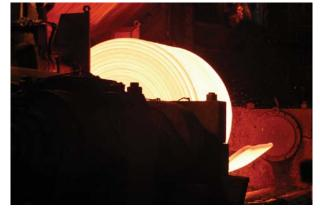
Fig. 1. Super Bainite sheet under production†
