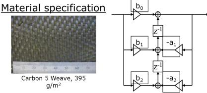
Figure 2 - Carbon fibre woven structural material and the novel digital filter architecture of the material implemented in the numerical model in the HIRF-SE Framework [19, 110].
