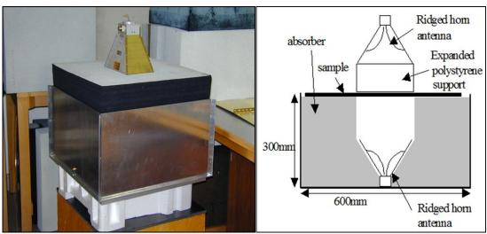
Figure 1 - Image and cross-section of the contactless SE measurement system [5].
