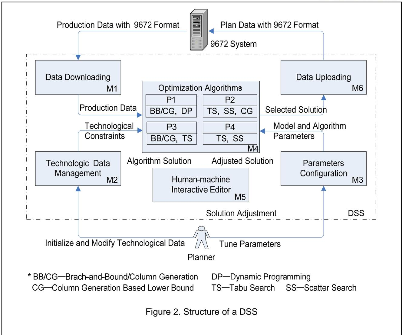
Figure 2. Structure of a DSS
