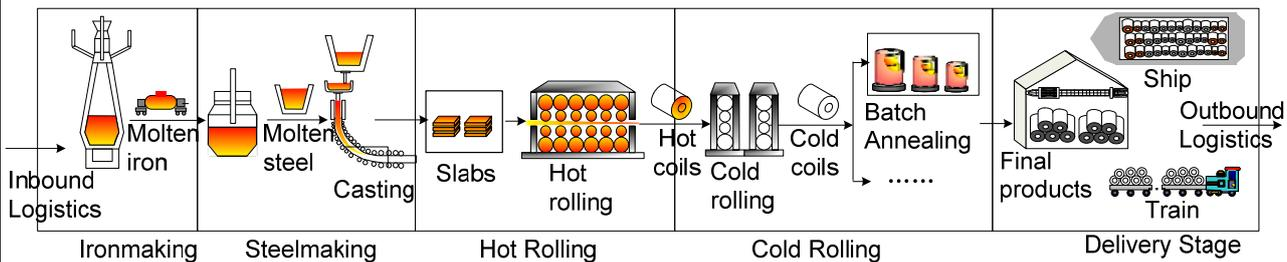
Figure 1. Stages of steel production and logistics system
