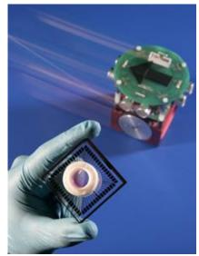
'Gordon', the mobile robot that wirelessly embodied a brain cell culture grown on a multielectrode array (in close-up).
