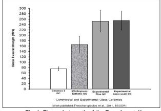
Fig. 1: Flexural strength of the Experimental/ Commercial glass-ceramics
