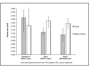
Fig. 2: Wear of the Experimental/ Commercial glass-ceramics
