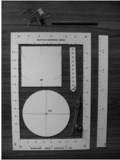
**Working principle of TGT:** TGT works on a simple principle that *when a stylus or sharp pen is pressed on a 'German film' placed on a soft rubber backing pad, raised lines are produced.* ('German Film' is a translucent and lightly textured polymer sheet. A touch-detectable raised line forms when drawn upon with a simple scribe or ballpoint pen on a soft rubber-backing pad).
