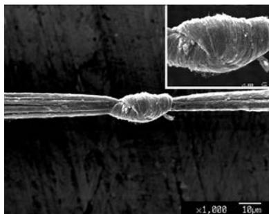
**Figure 1.** A tight knot in the tough CNT fibre. The knot does not fail prematurely under tension.
