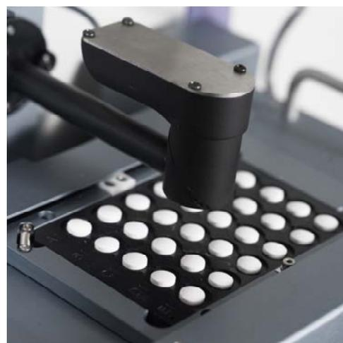
**Figure 1** High throughput drug analysis-tablets being analysed in a Raman spectrometer as used in FSNI
