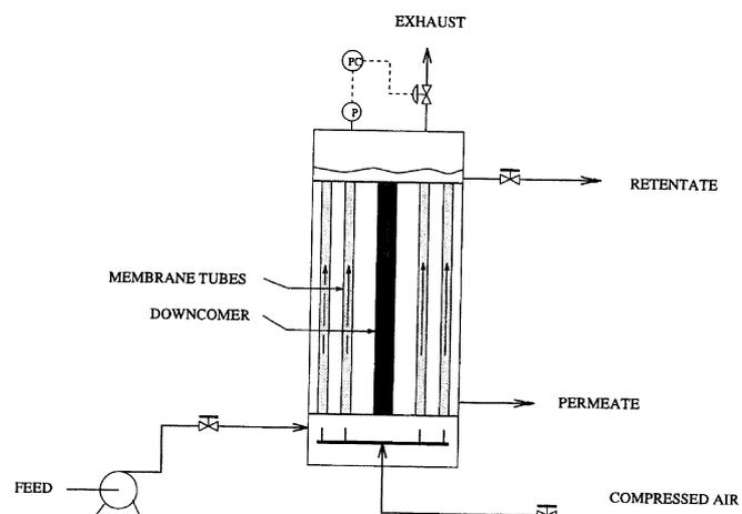
*Fig. 3: Air-lift gas-liquid two-phase cross-flow filtration.*
