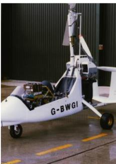
Original straight keel. When the propeller size increased it was necessary to raise the height of the propeller to avoid the keel – this introduced instability.
