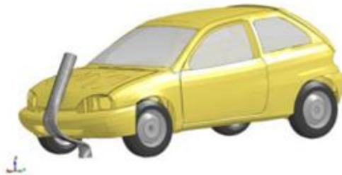
Figure 2: Finite element simulation of whole car crashing against sign post
