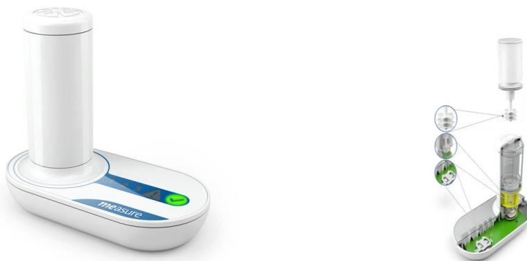
**Figure 1:** ModeDx, Left, measure® BOWEL HEALTH is a hand-held biosensor for measuring faecal occult blood; Right, schematic showing an exploded view of the faecal sampling interface to the biosensor device.
