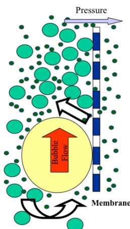
*Fig. 1: Gas-liquid cross-flow membrane filtration.*
