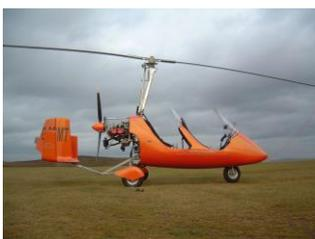
Dropped/stepped keel introduced as a result of the University of Glasgow recommendations to CAA, adopted in BCAR Section T. The dropped keel enables the propeller to remain low, maintaining stability. (Image courtesy of RotorSport UK Ltd)
