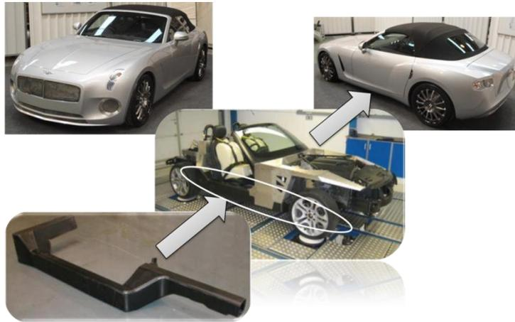
Figure 2: carbon fibre chassis rails manufactured using the Raycell concept and its location on the Bentley T35 demonstrator vehicle
