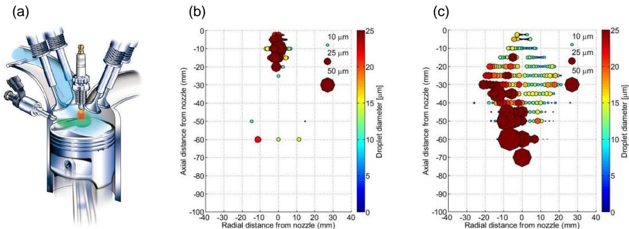
**Figure 1. Examples of 'instantaneous' characterisation of a Pressure-Swirl GDi Spray**
