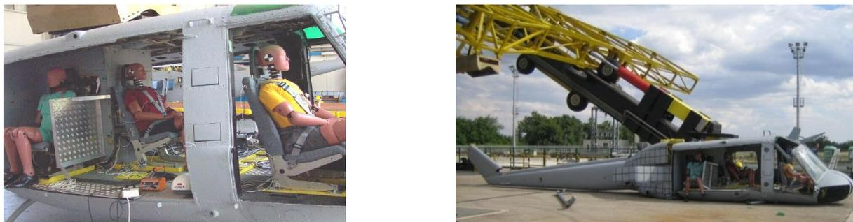
Figure 2 Helisafe Crash Test Dummies and Helicopter Crash Structure
