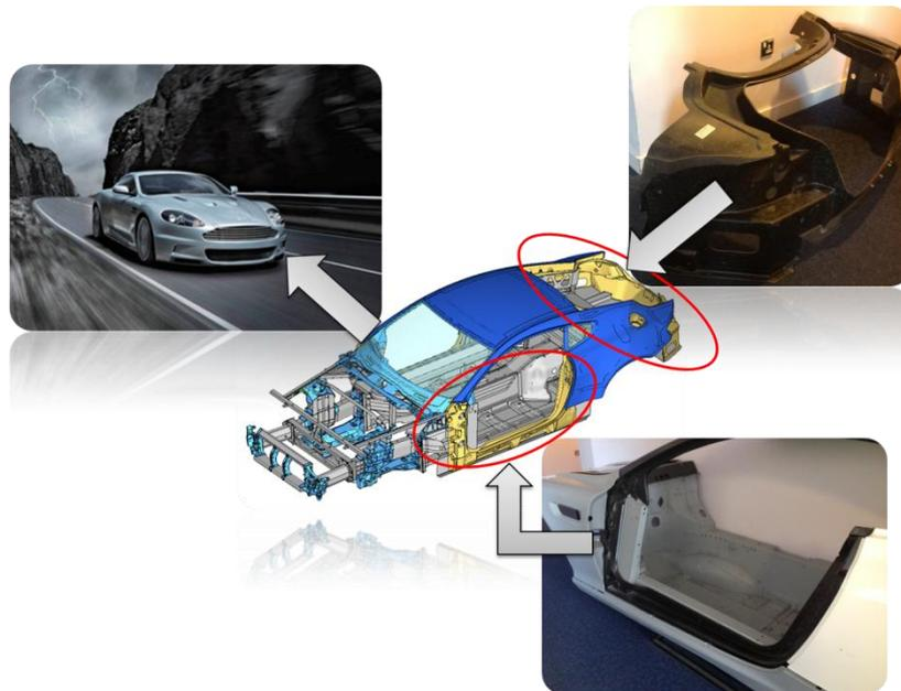
Figure 1: showing carbon fibre parts manufactured using DCFP and their location on the automobile
