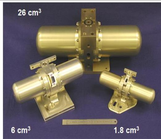
*Cryocoolers of different sizes*
