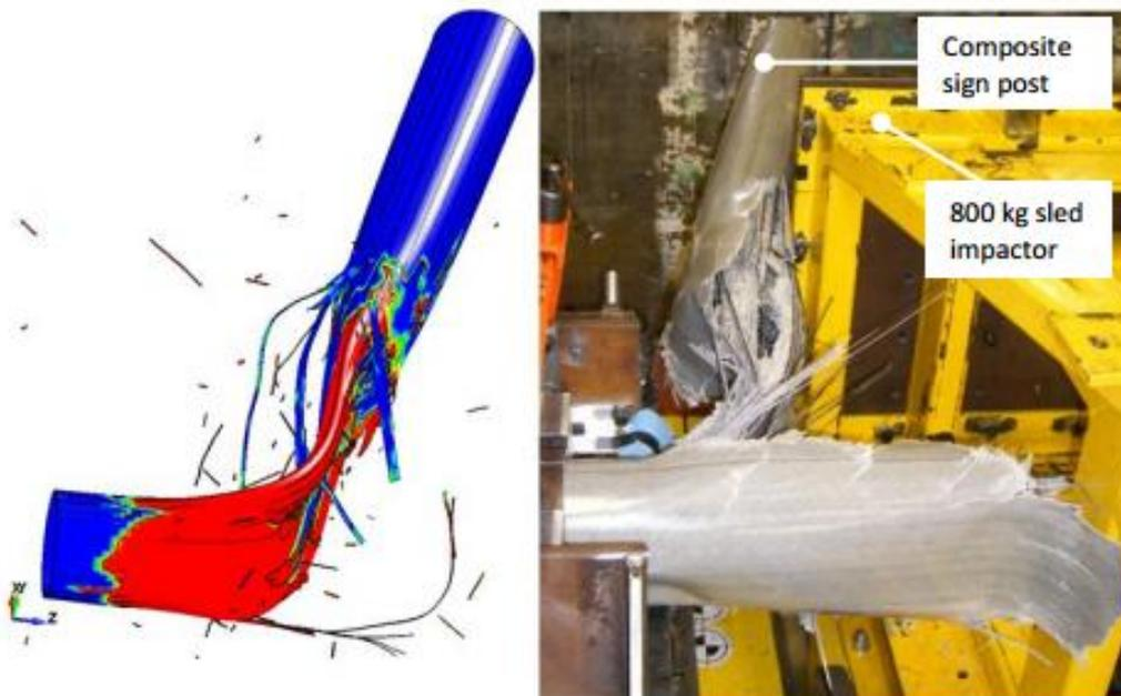
*Figure 1: Finite element model showing material behaviour of sign post under crash conditions (left); Physical crash test of same material performed at UoN labs (right). Note: excellent replication of model by physical test.*
