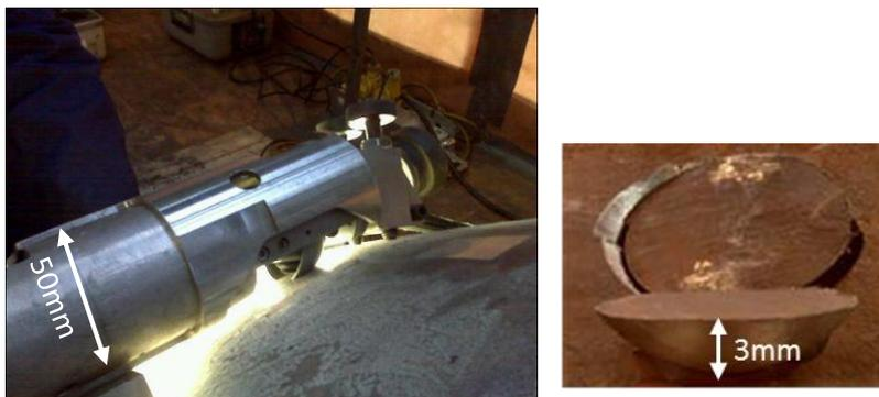
*Figure 1: Scoop sampling in progress (left), extracted scoop sample (right)*
