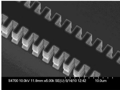
**Figure 1.** Lateral grating on the side wall of a QCL.
