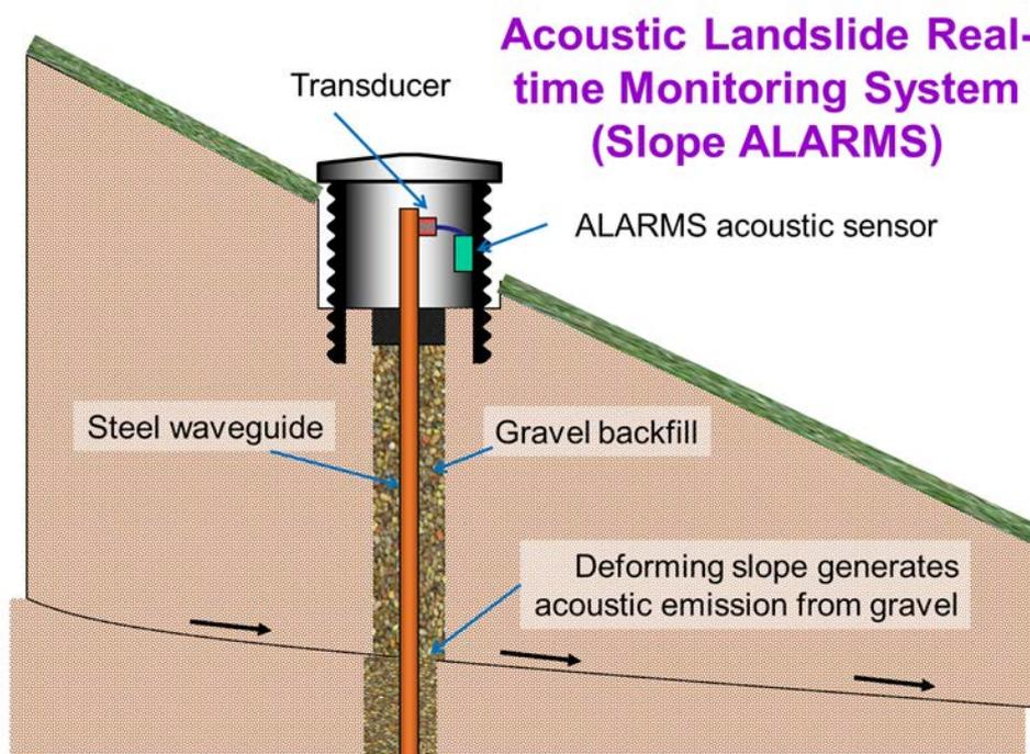
Figure 1: Slope ALARMS arrangement
