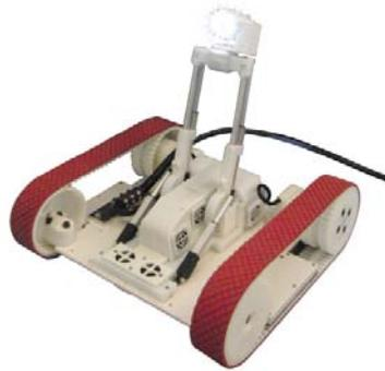
Fig 5: radio controlled wall climbing vehicle with GR1
