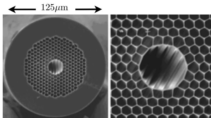
The cross section of a hollow-core PCF developed at Bath
