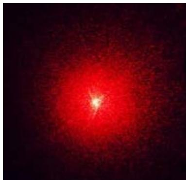
Fig 2: Laser speckle pattern from surface roughness
