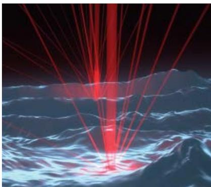
Fig 1: Surface roughness giving rise to diffuse light
