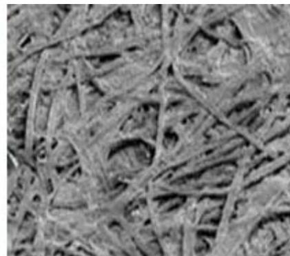
Fig 3: Electron microscope image of paper fibres
