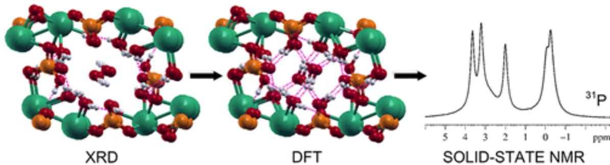
Fig 1. Example CASTEP output exploring biomineralisation of octacalcium phosphate (OCP), a precursor phase in bone mineral formation. This shows X-ray crystallography, first-principles density functional theory calculations, and solid-state nuclear magnetic resonance spectroscopy predictions of the structure.
