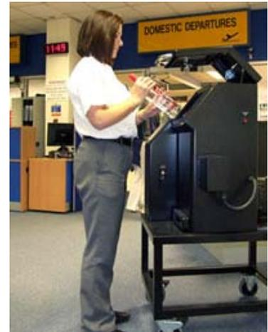
Fig 3. Bottle scanner in use in airport security
