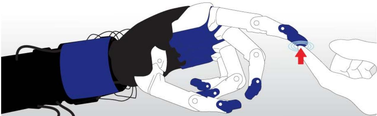
Fig 3: Tactile human-machine interface with QTC skin developed for robotics with NASA and MIT
