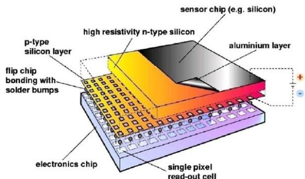
**Figure 1:** A picture and schematic diagram of the high-sensitivity, low-noise Medipix2 chip.
