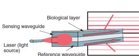
Fig 1 Schematic design for the instrument with silicon oxynitride layer waveguides
