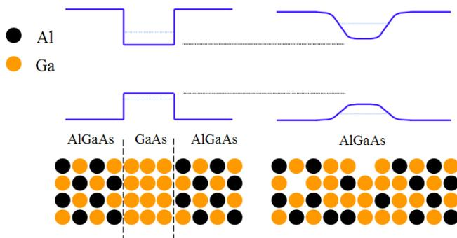
**Figure:** Illustration of band-structure and layer structure of a non-processed (left) vs. a QWI processed quantum well (right)
