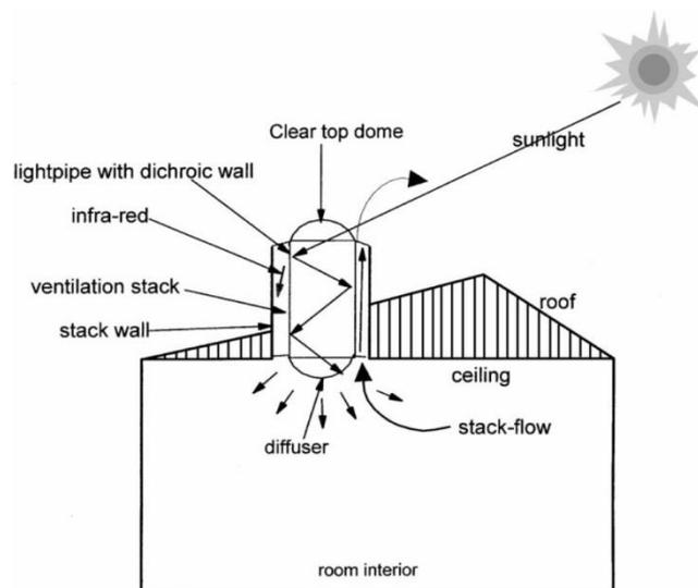
Figure 1: Illustration of Sola-Vent concept
