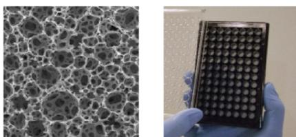
*Fig. 1 Scanning electron micrograph of Alvetex<sup>®</sup> scaffold (left). Example of a 96-well plate product containing Alvetex<sup>®</sup> 3D culture technology (right).*
