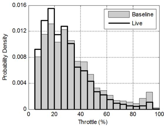
Fig. 1: Accelerator pedal (throttle) activation probability density before (Baseline) and after Lightfoot® was activated (Live). Note the shift towards lighter pedal activation when the device is active. Fuel use is proportional to accelerator pedal position.
