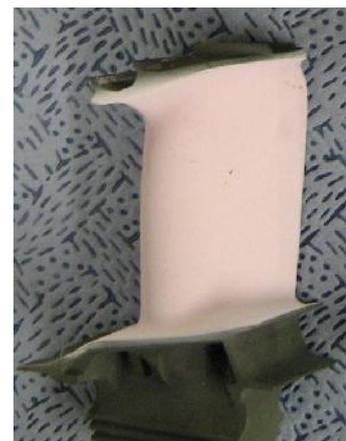
Figure 1: An aerofoil coated with a low K thermal barrier doped with Erbium at Cranfield
