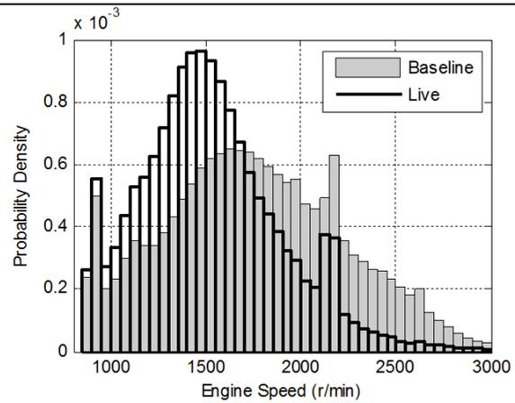
Fig. 2: Engine speed probability density before (Baseline) and after Lightfoot® was activated (Live). Note the considerable shift towards lower engine speeds when the device is active. Lower engine speeds are typically more efficient for an equivalent power output due to reduced friction.
