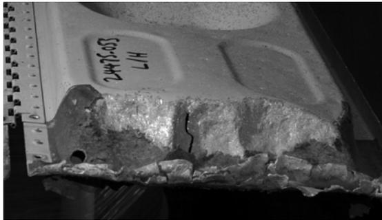
*Fig 1 Runway debris damage to the leading edge of an undercarriage door of a transport aircraft*
