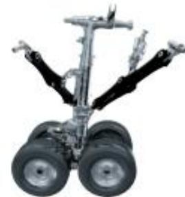
*Figure 2: Detail of the landing gear of the Boeing 787 (the composite braces are shown in black).*
