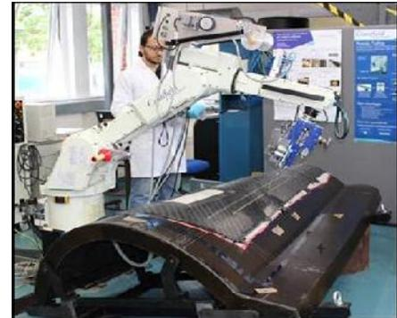
*Figure 3: Tufting robot at Cranfield inserting tufts in a double-curvature surface.*
